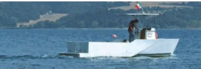
Figure 7b (below) – 14 knots on the 8.1 metre model corresponding to 23 knots for a MonoTriCat® with a water line length of 21 metres. Despite travelling at the top end of semi-planing speeds the wave formation is contained and the trim remains practically horizontal.
