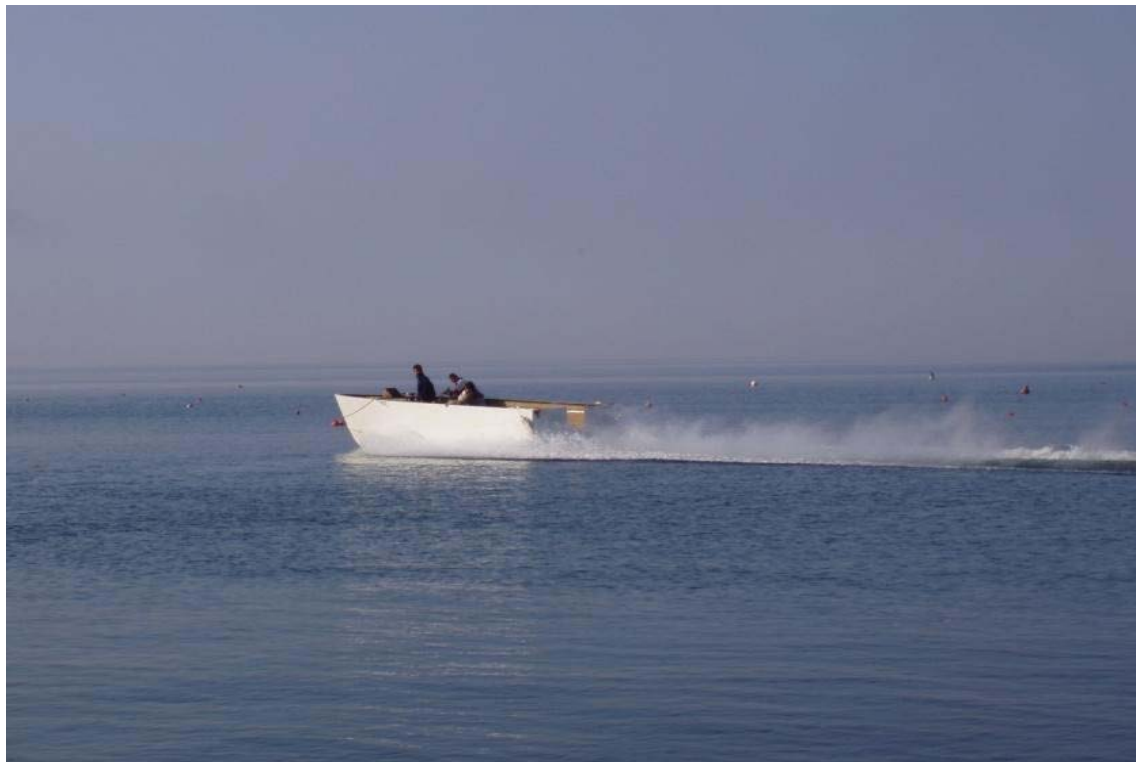
Figure 5. Self-propelled model hull navigating on Bolsena Lake (speed 22-24 knots)
