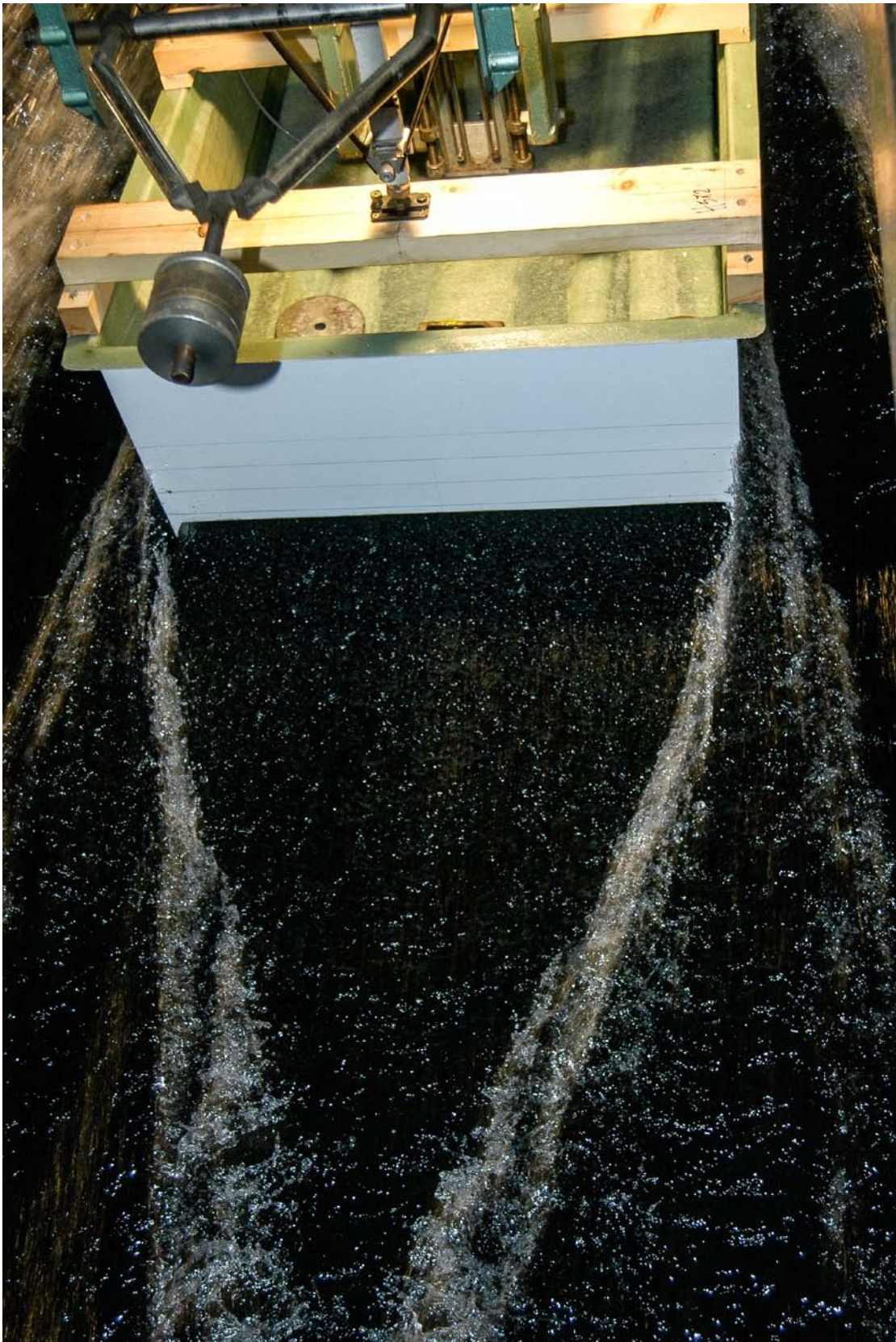
Figure 7. Spray hull Test towing \Delta 70t - speed 24 knots, Towing Tank INSEAN CNR Rome, 2010.
