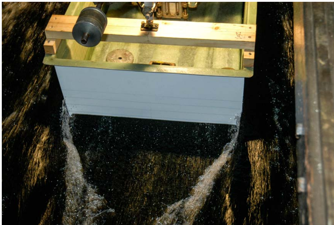
Figure 6. Spray hull Test towing \Delta 70t - speed 18 knots, Towing Tank INSEAN CNR Rome, 2010.
